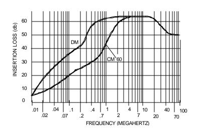
This EMI / RFI filter features a very small mechanical package. Even with this small size the common mode insertion loss and differential loss are more than is available in other similarly sized packages.
